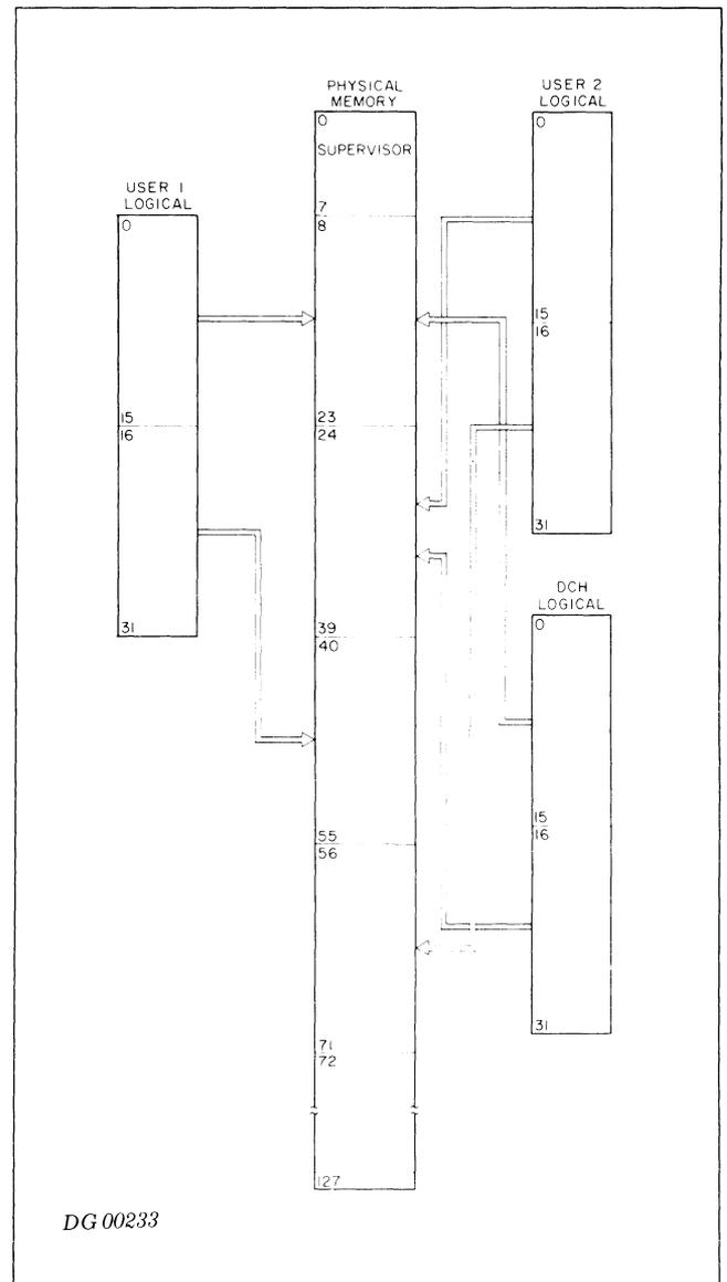
In order to manage memory efficiently, the operating system makes use of the validity and write protect features of the address translation hardware, if possible. The next figure shows a two-user configuration where these features are used.
