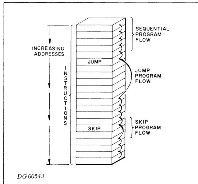
Because the program counter is 15 bits in length, it can address 32,768 separate memory locations. The next memory location after  $77777_8$  is location 0, and the location before 0 is location  $77777_8$ . If the program counter rolls from  $77777_8$  to 0 in the course of sequential operation, no indication is given and processing continues with the location addressed by the updated value of the program counter.
