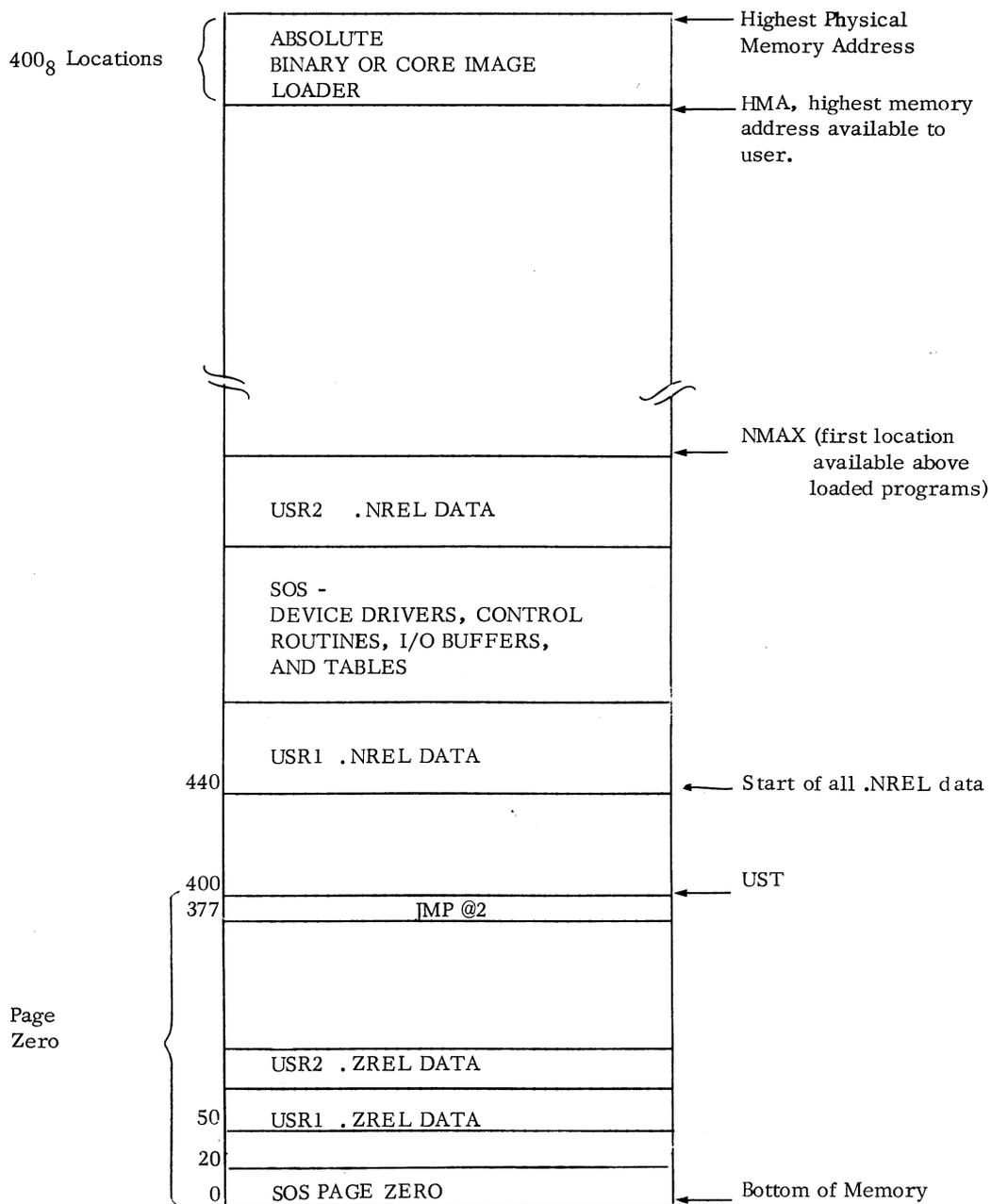
Figure 1-1. Loaded Program in Core
