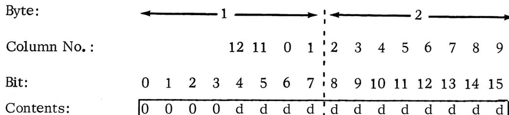
The "d's" will be 1 for every column punched. End-of-card in a read sequential is signified by a byte pair containing the word 100000. The specified byte count must be an even number.
