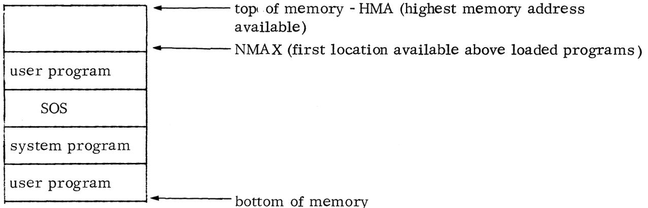
The highest memory address available (HMA) is usually the first word below the Binary or Core Image Loader.
