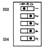
Switch is shown with Position 2, 3, 4 and 5 ON which equals Device Code Selection of 40, 41.
