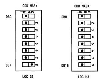
DBO = Data Bit 0, DB15 = Data Bit 15, Mask Bit 7 shown selected
