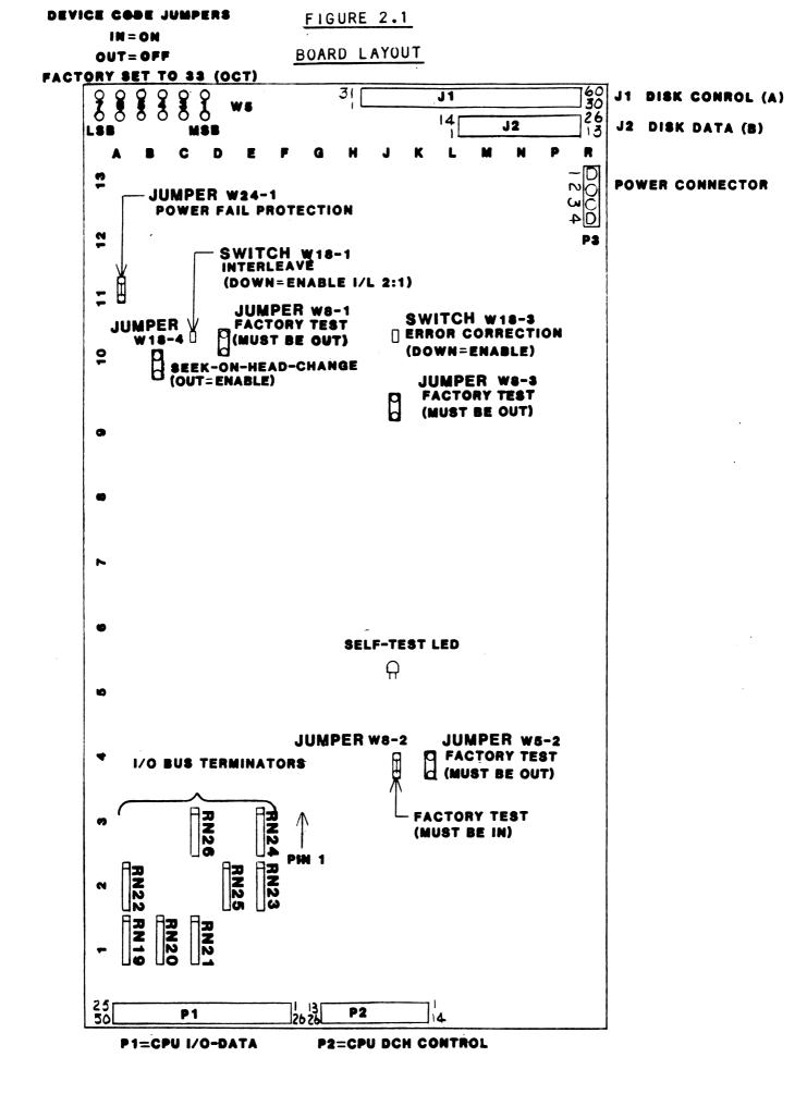
The following sections provide further information on individual board setup options. Some of the jumpers used are actually miniature switches mounted on .1" centers. The switches contain high-tension locking contacts that open and close by pulling up and pushing down on the switch center.
