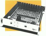
Allows processors, one at a time, to access the peripheral requested. Interfaces to Zetaco's BMX-2 and TC-133 Tape Couplers, and our LPC-3 Printer Controller.
