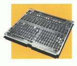
16-channel programmable multiplexor supports 16 user consoles on a Nova or Eclipse system. Operates in the CPU chassis, with or without DCU. Sup-
